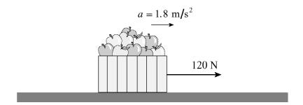
Find the coefficient of friction between the carton and the ground.
