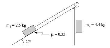
a) Find the acceleration of the system of masses.
