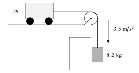
If this system accelerates at  $3.5 \text{ m/s}^2$ , what is the mass m of the cart?
