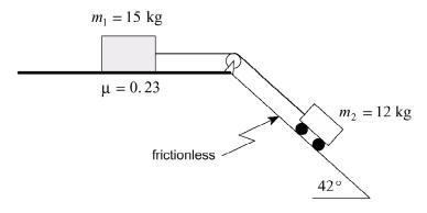
Determine the acceleration of the system of masses.
