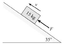
What minimum force F, would be necessary to move the block up the incline at a constant speed?
