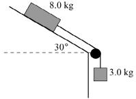
What is the acceleration of the 8.0 kg block down this ramp?
